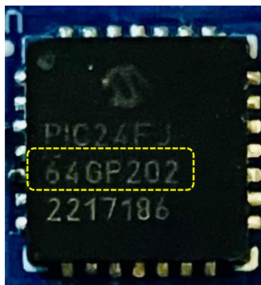
Appearance of the PIC24FJ64GP202 Processor on Backside of M3-L Module at U1
