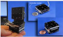
M3-LS Linear and M3-RS Rotary Stages can be assembled into multi-axis motion systems. With a controller embedded in each stage, these systems eliminate the need for bulky external control boards. They deliver the smallest system size and fastest integration for precision, closed loop motion in two or three axes.
