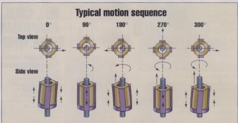
In Squiggle motors, piezoelectric actuators create ultrasonic vibrations in a tube, which makes a threaded nut at the end of the tube vibrate in an orbital fashion. The nut threads onto a screw shaft, translating the orbital motion into linear motion of the screw. Drive signals 90° out of phase with each other drive two sets of piezo actuators to produce the orbital motion. Reversing the phase relationship lets the device move the shaft in the opposite direction.
